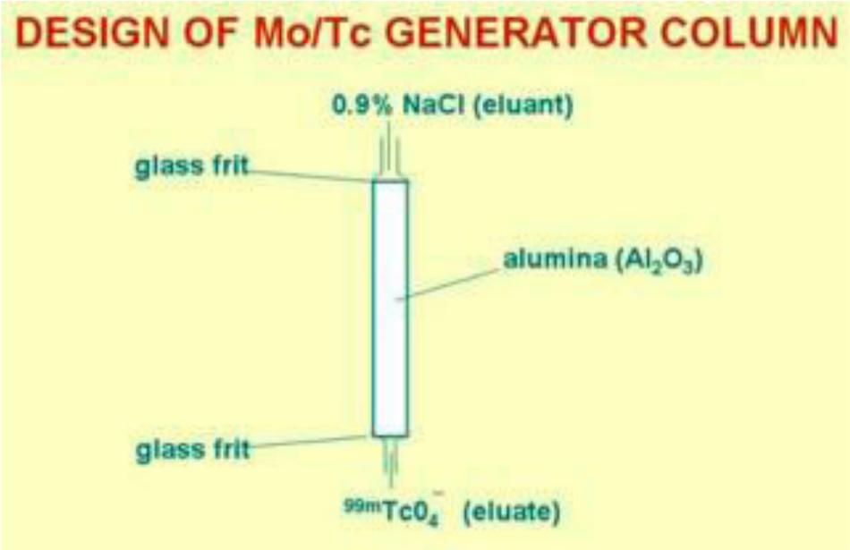
**Mo/Tc Generator: Schematic of A Dry Column Generator-Internal Construction**
